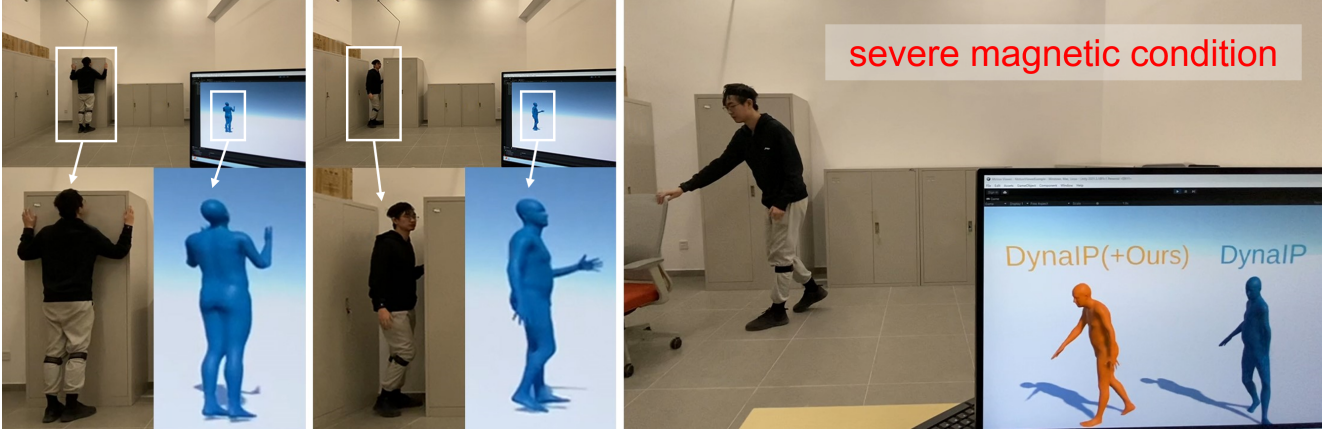
Figure 1. We propose MagShield, an IMU orientation estimation method that specifically designed to address magnetic disturbances in sparse inertial MoCap systems. By integrating with our method, existing sparse inertial MoCap systems (left, PNP; right, DynalP) can operate reliably even under severe magnetic condition.
