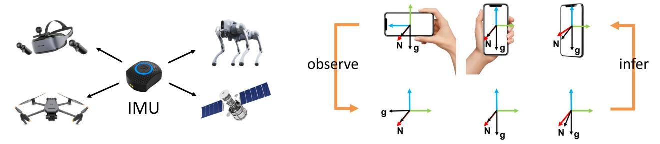
How magnetic disturbances affect IMU? IMUs can be misled by "fake north". Since pitch and roll can be inferred from gravity, only <u>yaw error</u> remains.
